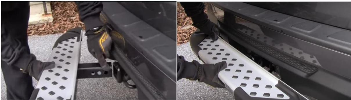
**Step 3:** Install special bolt, using a 22mm socket or wrench tighten bolt until hitch does not move. Install safety pin, you have completed the installation.
