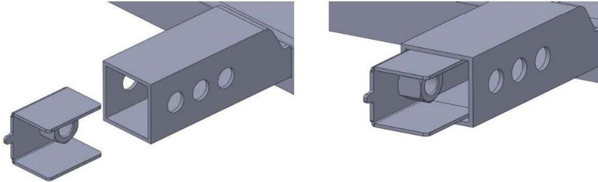
**Step 2:** Slide hitch step into 2-inch receiver. Make sure to choose one of three positions.
