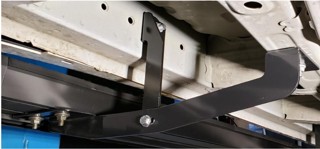
Image shows pass front bracket installed
