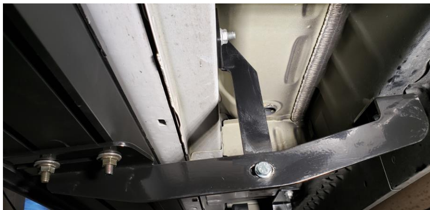
Image shows pass middle bracket installed
