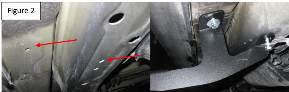
**Step 4:** Install rear bracket with provided hardware. Note you must enlarge outer hole to 1/2 inch in order to install provided M8 special nut. Install bracket as per Figure 3. Do not tighten.
