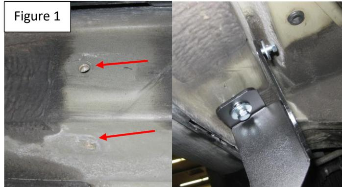
**Step 3:** Install middle bracket with provided M8 hardware Figure 2. Do not tighten
